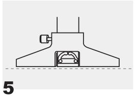
Once installed, check the depth base to be sure it is on the same plane as the end of the caliper.
