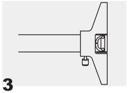
Align the base with the bottom of the caliper.
