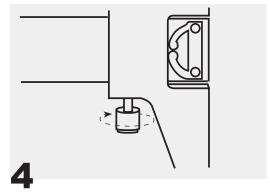
Tighten the tumb screw to keep it in place.
