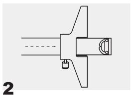
Slide the depth base forward, keeping pressure on the base and spring clip.
