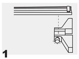
Loosen the thumb screw and install the depth base.
