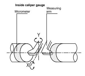
Calibrate the origin with gage block (for outside caliper gauge) or outside micrometer (for inside caliper gauge) before measuring. Clean measuring faces of gage block or outside micrometer and measuring
